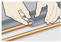
(including cold water pipes) to reduce idling losses. For a snug fit, match the pipe insulation sleeve's inside diameter to the water pipe's outside diameter, and tape or cinch pipe insulation with cable ties every 1-2 feet. On gas water heaters, keep pipe insulation at least 6 inches away from the exhaust flue.
