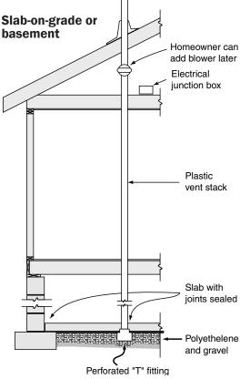
Slab foundation with passive radon-resistant technique
