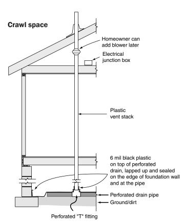
Crawlspace with passive radon-resistant technique
