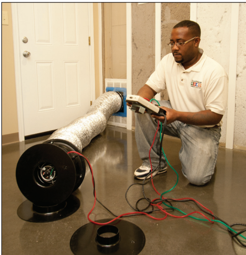
This technician is performing a duct leakage test that ensures the integrity of the duct system.
