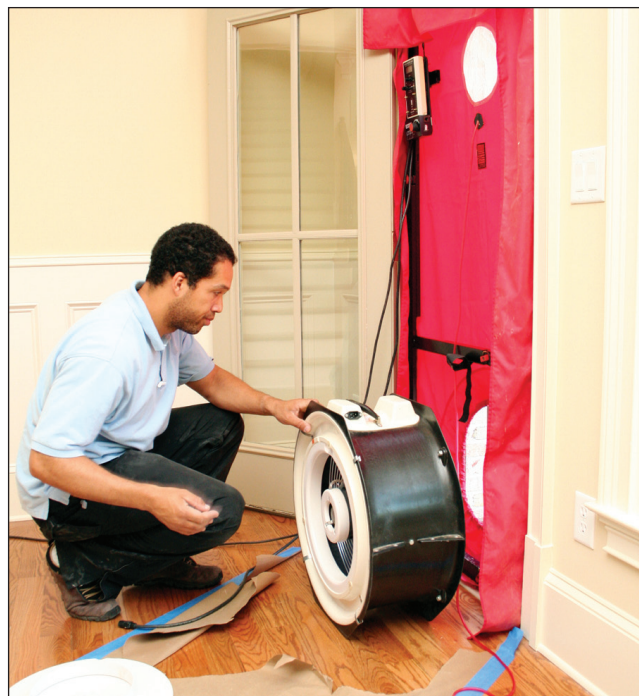
Blower door diagnostics indicate the level of "tightness" of a building. This helps determine air leakage of the building and pinpoint areas for sealing.
