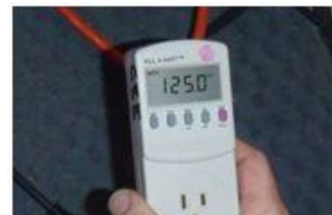
Before fan is turned on the meter reads 125 volts
