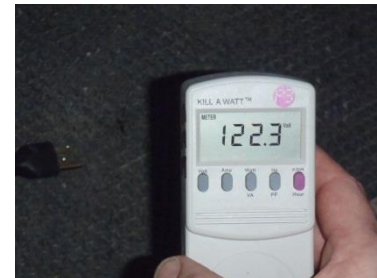
After fan is turned on the meter reads 122.3 volts, indicating that both outlets are on the same circuit
